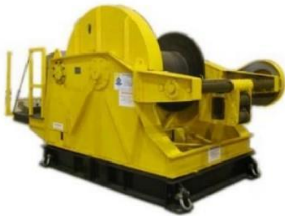
Figure 2-15: Typical shore based winch arrangement.
